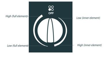
Fig.10 Dual element control knob (knobs may vary) (CT5602F & CT6551S models only)
